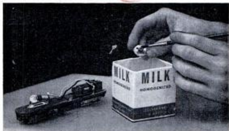
Cutting down a milk carton to a height of 2 or 3 in. provides a neat, throwaway holder for solvent when cleaning small parts
